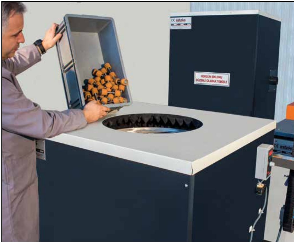
The Smart Feeding System with Double Magazines
