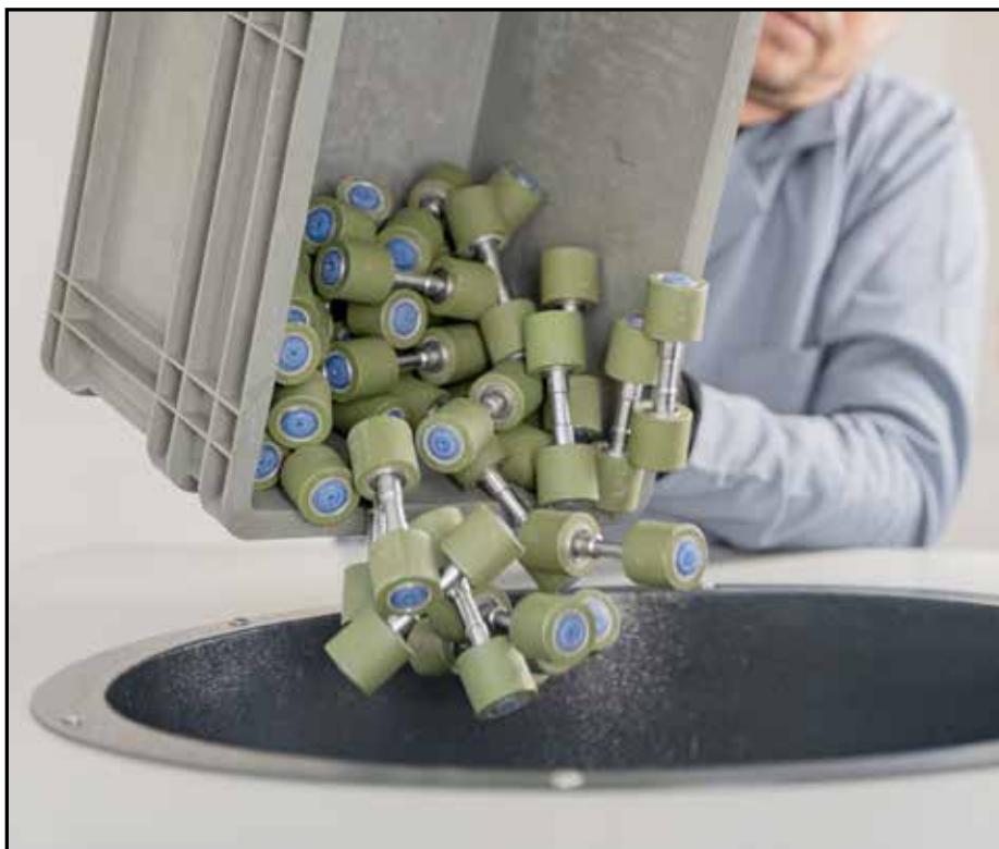
The Smart Feeding System with Magazine
