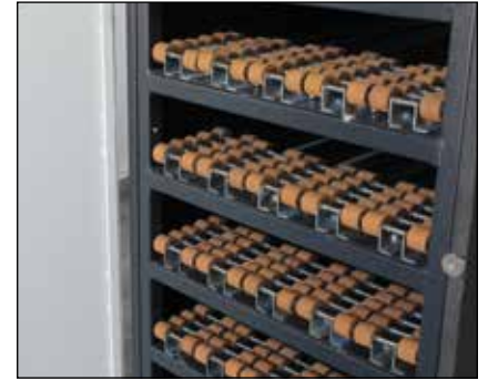
Top rollers carriage inside view.
