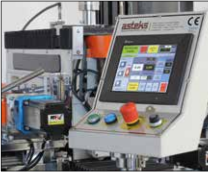
HMI Control Panel
